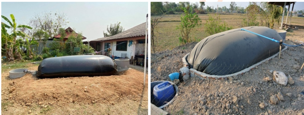
Fig. 2: Semi-continuous feed pilot scale of anaerobic biogas bag used in this study.
