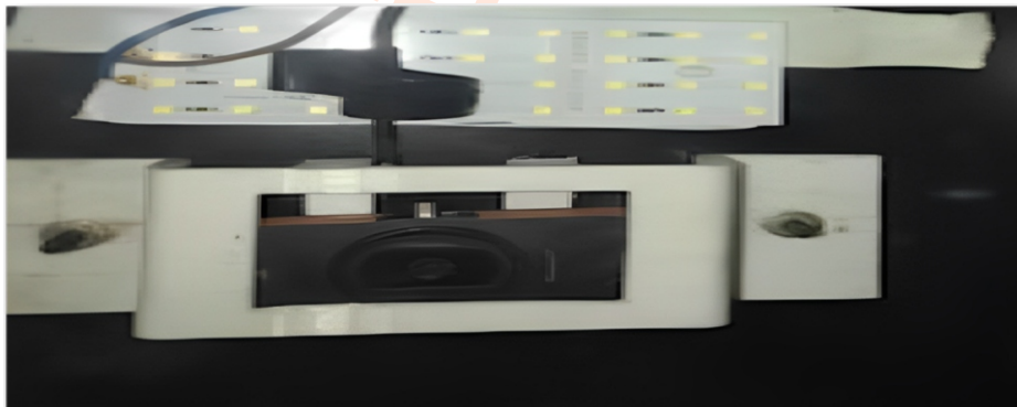
Fig. 5: Camera set up to detect the deterioration process of the commodity during storage.
