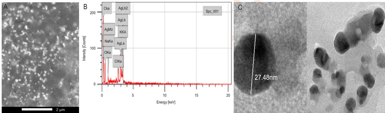
**Fig. 4:** Characterization of *Panibacillus* sp. NS-36 mediated AgNPs: (A) SEM analysis of NS-36 AgNPs; (B) EDX analysis of NS-36 AgNPs and (C) TEM micrograph of NS-36 AgNPs.
