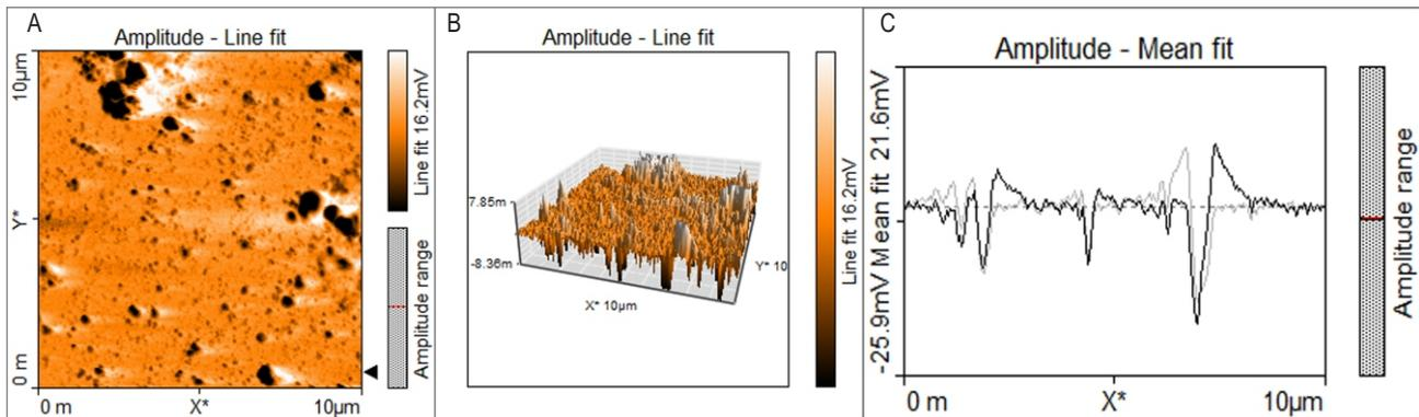
**Fig. 3:** AFM analysis of *Panibacillus* sp. NS-36 mediated AgNPs: (A) 2D structure of NS-36 AgNPs; (B) 3D structure of NS-36 AgNPs and (C) Particle size distribution of NS-36 AgNPs.
