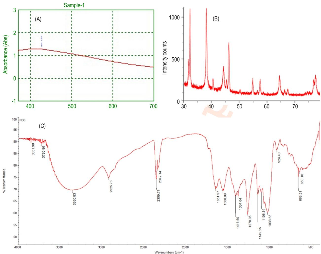
**Fig. 2:** Characterization of *Panibacillus* sp. NS-36 mediated AgNPs (A) UV-Vis spectra of NS-36 AgNPs; (B) XRD pattern of NS-36 AgNPs, and (C) FTIR spectrum of NS-36 AgNPs.
