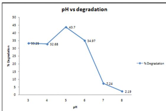
Fig. 11 : pH optimization for Acid Violet 4BY dye degradation using laccase enzyme
