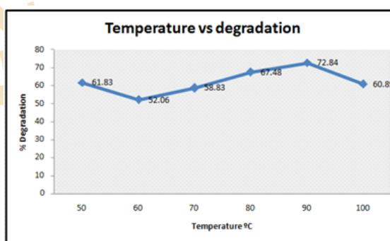
Fig. 16 : Temperature optimization for Direct Blue E dye degradation using laccase enzyme
