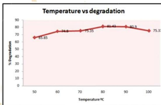
Fig. 14 : Temperature optimization for Acid Violet 4BY dye degradation using laccase enzyme
