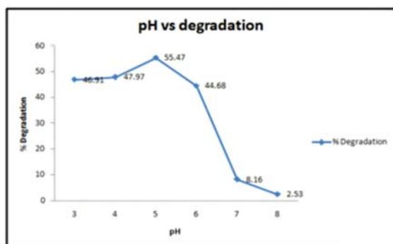
Fig. 13 : pH optimization for Direct Blue E dye degradation using laccase enzyme
