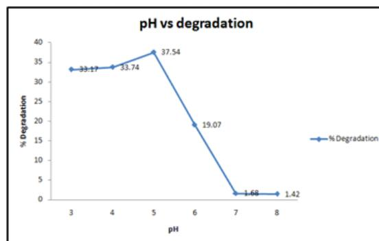
Fig. 12 : pH optimization for Acid Brilliant Black dye degradation using laccase enzyme
