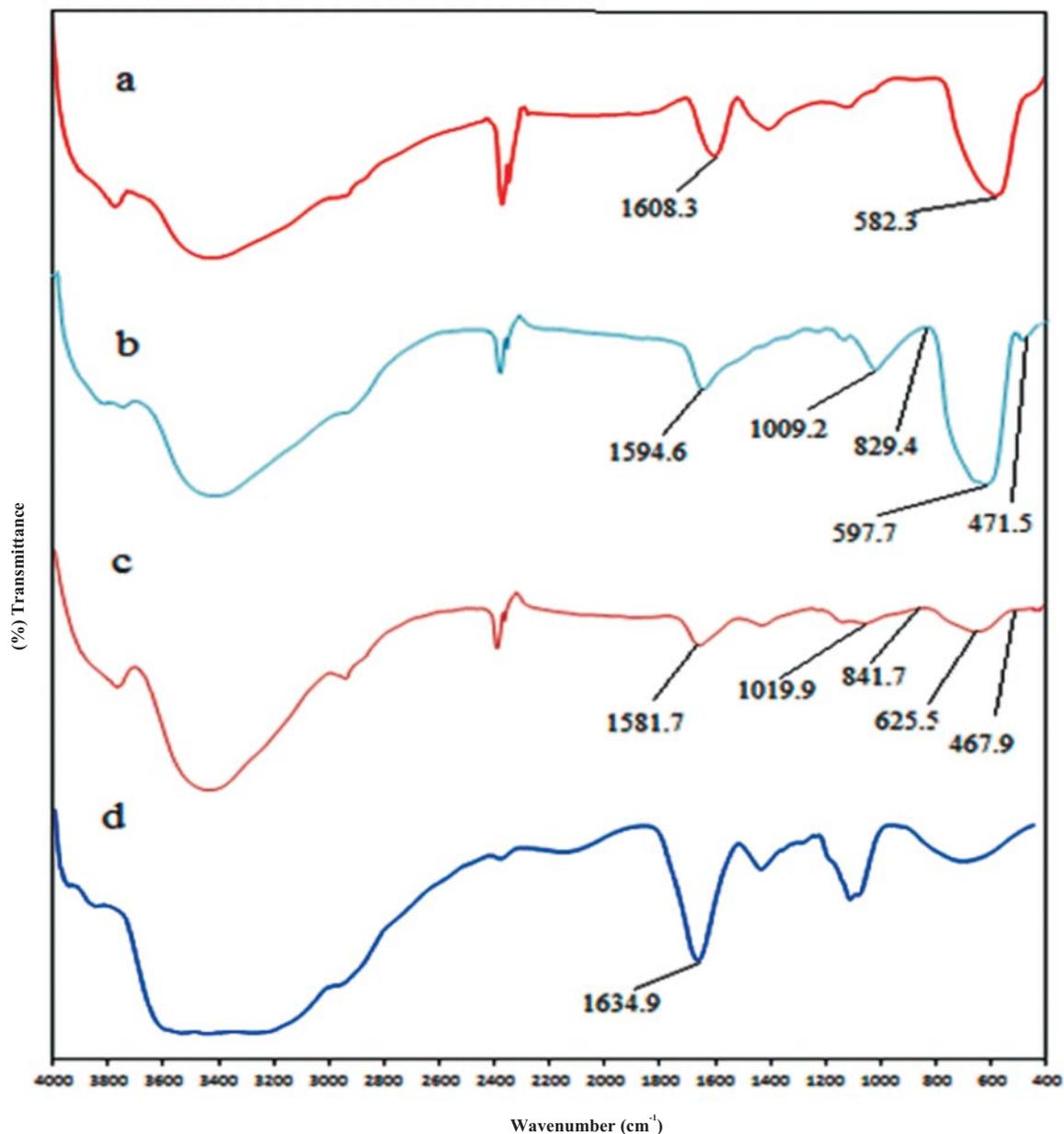
**Fig. 3 :** FT-IR spectra of (a) MNPs (b) AMNPs (c) laccase bound MNPs and (d) free laccase
