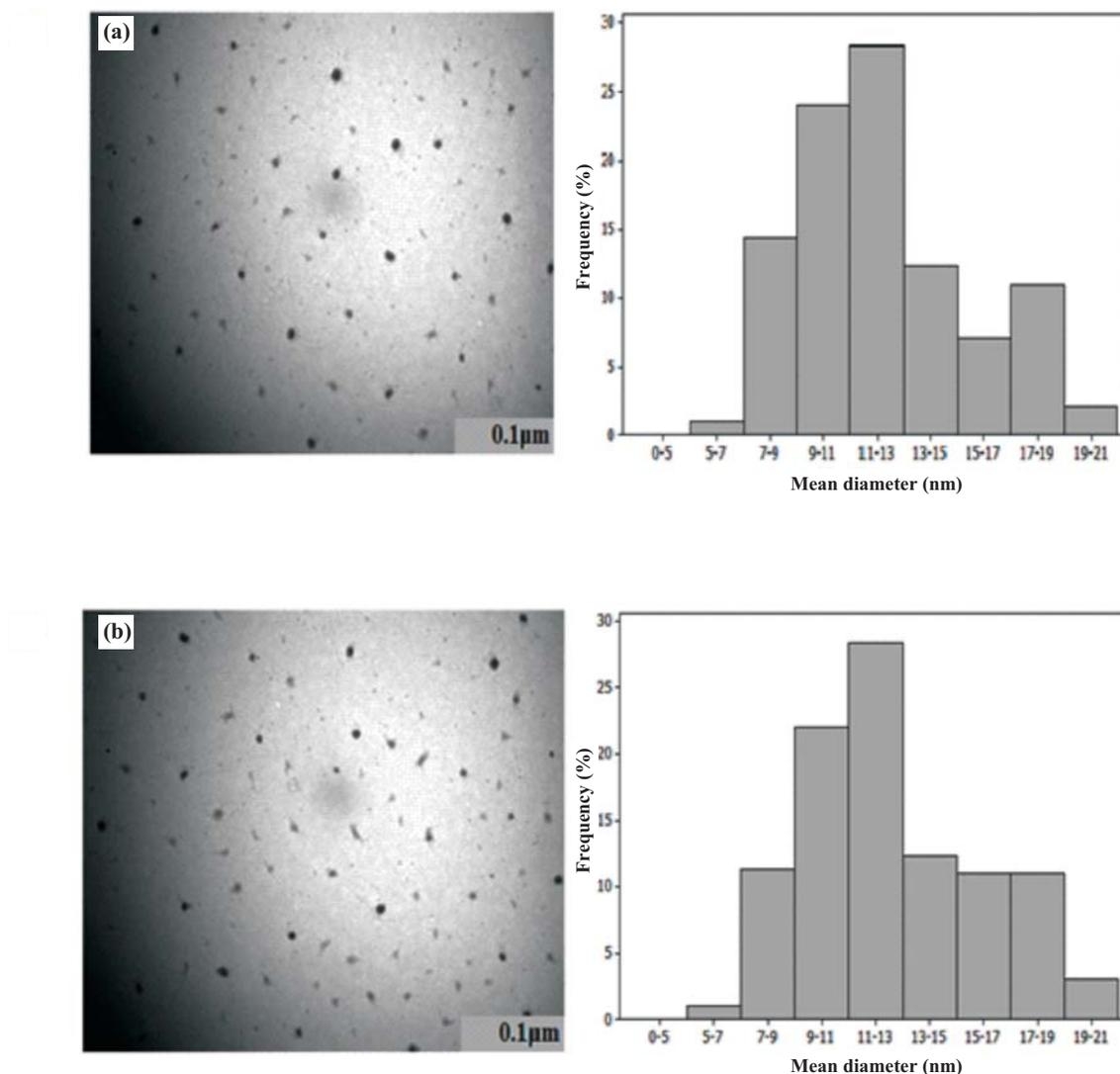
Fig. 1 : Micrographs and size distribution analysis of (a) naked and (b) laccase bound MNPs
