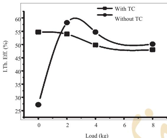
Fig. 1 : Load vs. Indicated thermal efficiency
