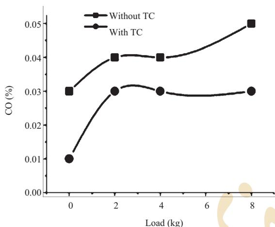
Fig. 5 : Load vs. Carbon monoxide
