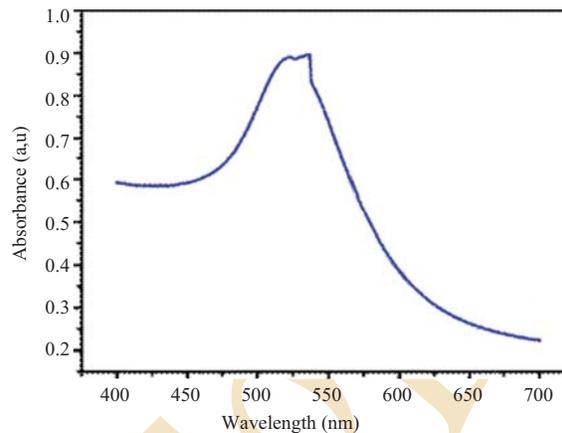
Fig. 1b : UV spectrometry of CGNP's
