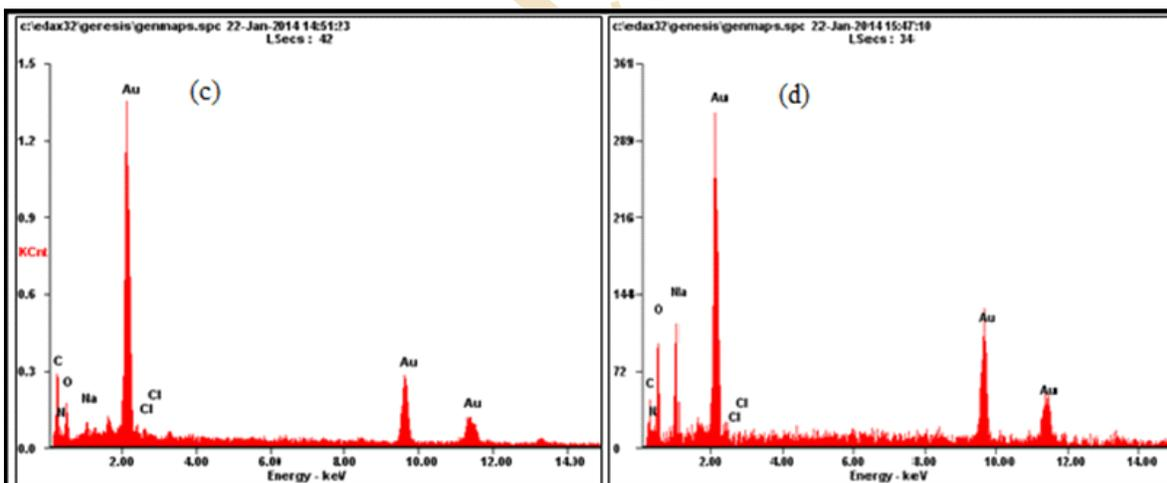
Fig. 2 : SEM image for a) BGNPs b) CGNPs c) EDAX spectrum for BGNPs d) is EDAX spectrum for CGNPs
