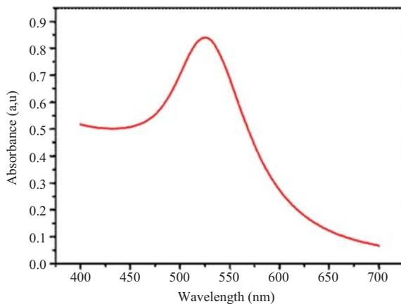
Fig. 1a : UV spectra of BGNPs
