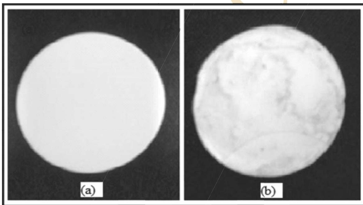
Fig. 6 : Visual observation of (a) uncoated membrane (b) AuNPs coated membrane
