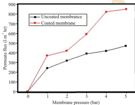
Fig. 8 : Variation in permeate flux with membrane pressure
