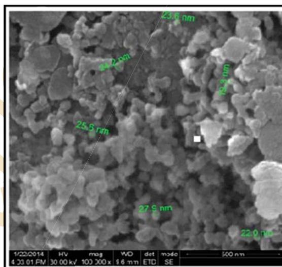
Fig. 3 : SEM micrograph of synthesized AuNps
