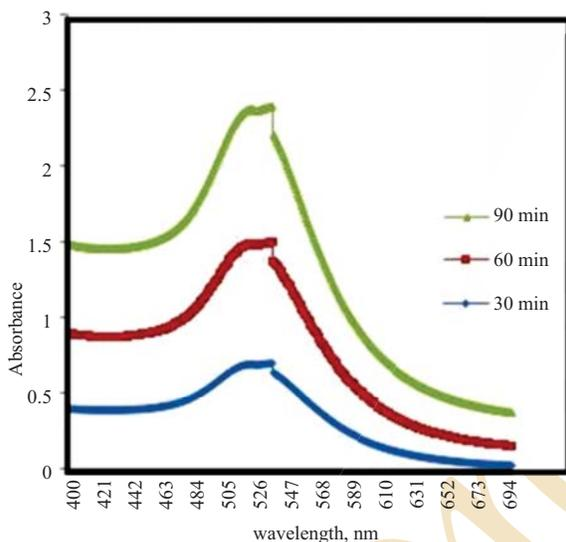
Fig. 2 : UV –Vis Spectrum of synthesized AuNps
