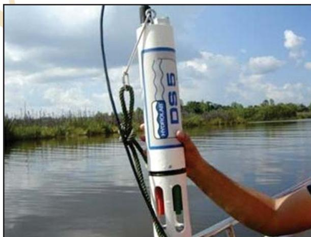
**Fig. 2 :** Surveying of Bera Lake water qualities by Hydrolab DS5 apparatus
