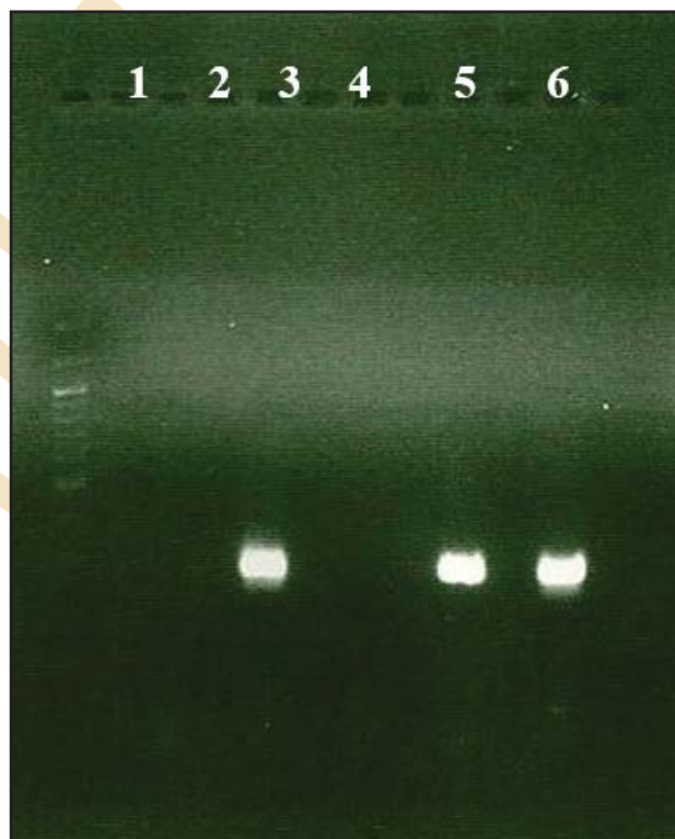
Fig. 2 : Salmonella spp. DNA cell results for samples that contained live cells, dead cells, and mixture of live and dead cells. Lane 1: Ladder (100bp New England Bio); Lane 2: Negative control; Lane 3: Positive control; Lane 4: 100% of dead cells of Salmonella spp.; Lane 5: 100% of live cells of Salmonella spp.; Lane 6: Mixture of 50% dead and 50% live Salmonella spp. cells.
