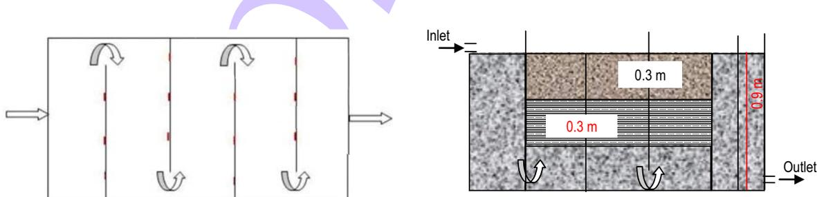
Fig. 1 : (a) Plan View and (b) Sectional View of Wetland Unit
