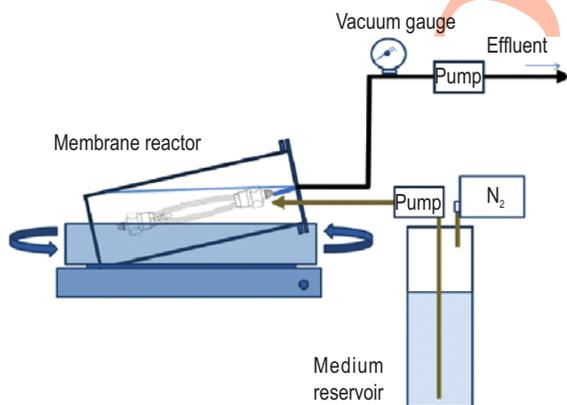
Fig. 1 : Schematic diagram of membrane reactors for inducing starvation
