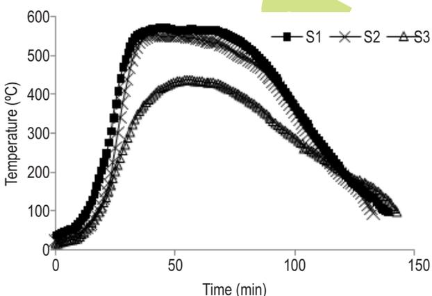
**Fig. 4** : Time/temperature profile of beehive briquettes made from charcoal-soil ratio of 60:40 (S<sub>1</sub>), 50:50 (S<sub>2</sub>) and 40:60 (S<sub>3</sub>)
