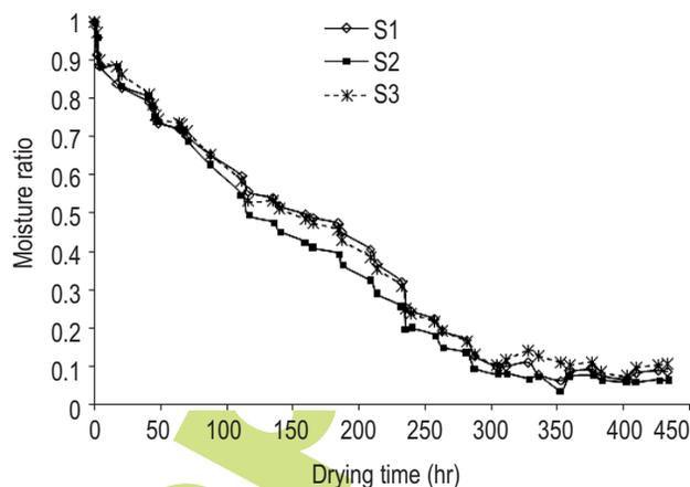
Fig. 2 : Natural drying curves of beehive briquettes made from charcoal-soil ratio of 60:40 (S<sub>1</sub>), 50:50 (S<sub>2</sub>) and 40:60 (S<sub>3</sub>)
