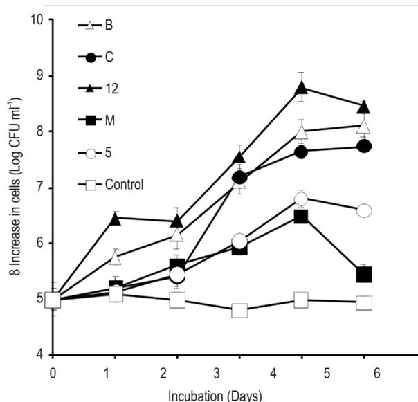
**Fig. 1 :** Growth curve of diesel-degrading isolates on medium supplied with 2.5% diesel incubated on an orbital shaker (150 rpm) at 30°C for 5 days. The bacterial growth measurement was based on colony forming unit (Log CFU ml<sup>-1</sup>). Value are mean of three replicates  $\pm$  SE
