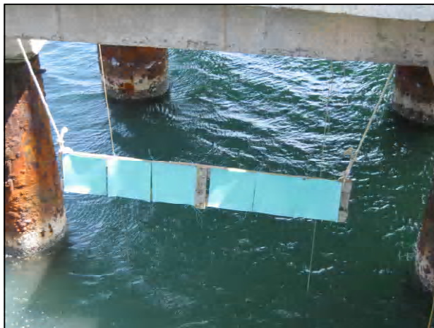
Fig. 1: Immersed PVC biofilm sheets on wooden rack
