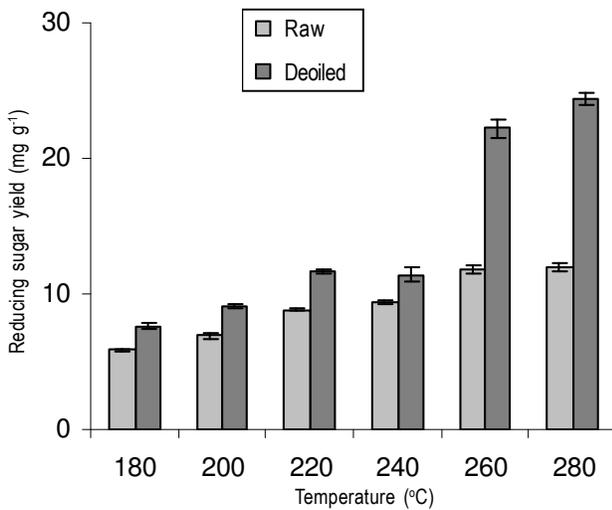
Fig. 1: Reducing sugar yield by subcritical water hydrolysis of raw and deoiled squid viscera at different temperatures
