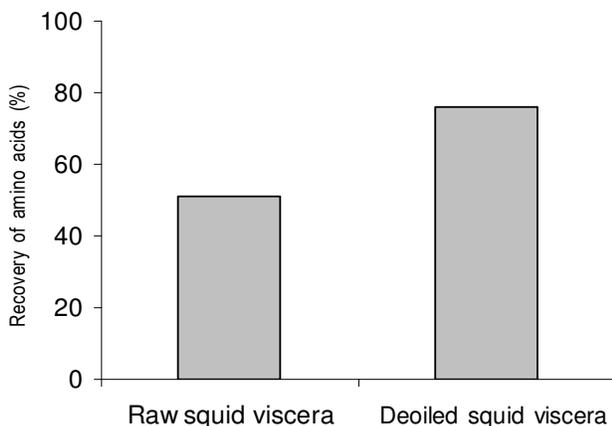
**Fig. 4:** Recovery of amino acids from raw and deoiled squid viscera by subcritical water hydrolysis
