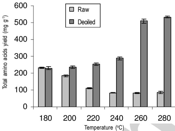
Fig. 2: Total amino acid yield by subcritical water hydrolysis of raw and deoiled squid viscera at different temperatures
