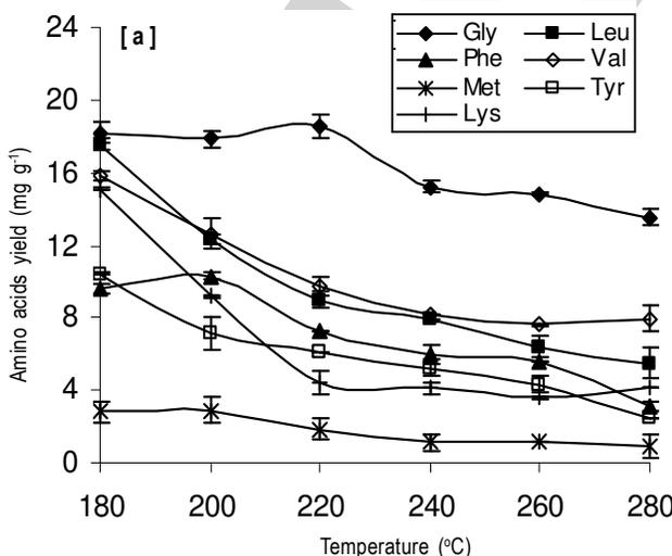
strong aggregation through hydrophobic interactions. However the solubility of protein in water increased at higher temperature. Moreover, the protein yield increased at elevated temperature was due to the increased rate of hydrolysis activity caused by the increase in dissociation constant or ion product constant of water.
