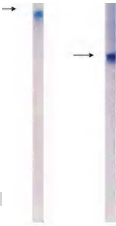
Fig. 1B: Native PAGE of affinity purified non-denatured lectins at pH 4.5 using 7.5% tube gels. 80 \mu\text{g} of each sample was loaded separately on each tube gel and electrophoresis was carried out using \beta -alanine-acetic acid buffer, pH 4.5 at a constant 150 V
