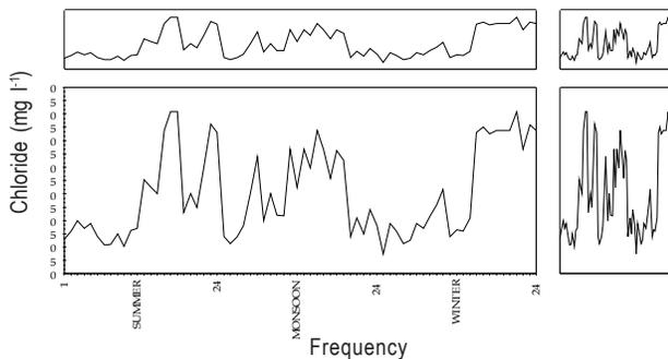
Fig. 4: Time series plot for temporal variation of chloride
